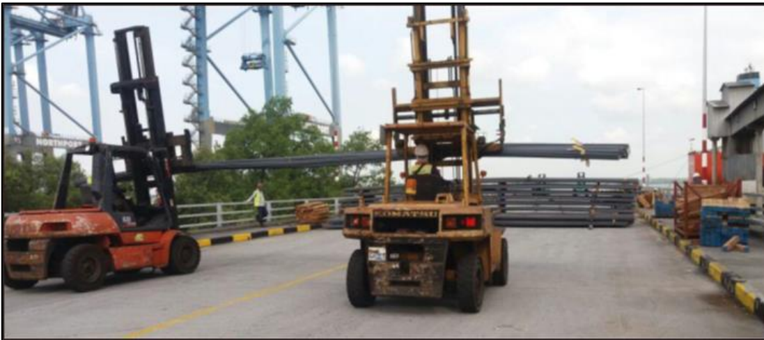
Diagram 4: 5-ton Forklift handling Long Length Cargo (40' bar cargo)
